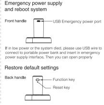
This procedure will delete all user codes associated with the lock. Use a needle to long press the reset button when the power is on. After hearing the voice prompt, please continue to press the key until restore the factory settings.
